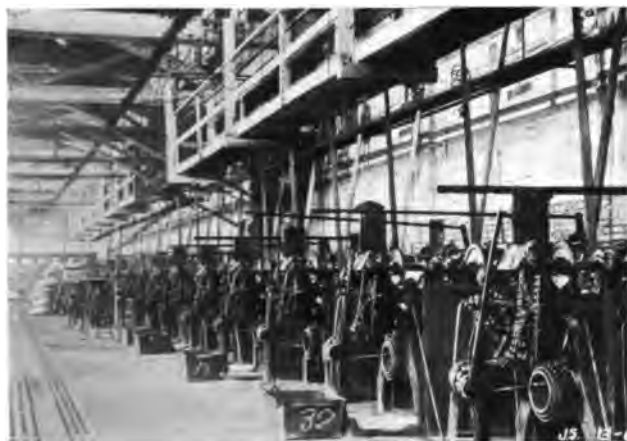
Fig. 4. Barbed Wire Fence Machines, before and after guarding.* Fig. 5.
